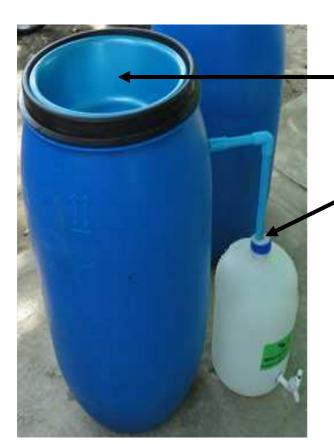
Remember to put a large cover over the top of the drum and drip bowl to stop dirt, dust and insects falling into the system.
